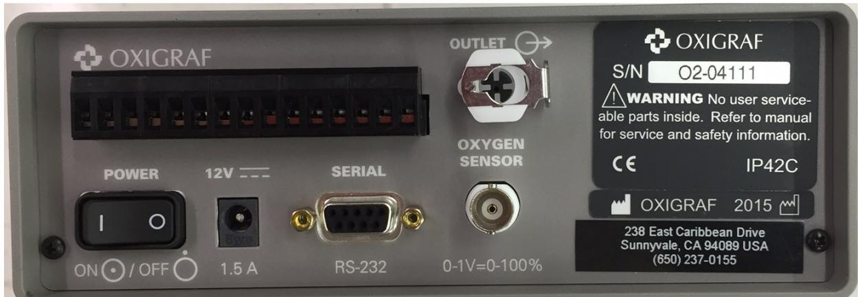
The power on/off switch (Press “I” for on, “O” for off), 12 VDC power input jack, service interface, terminal block interface, and a gas outlet port are located on the instrument back panel. Power is supplied by an external 12 Volt, 2 Amp CSA Level 3 power supply. The RS – 232 port is provided to interface with a computer.
