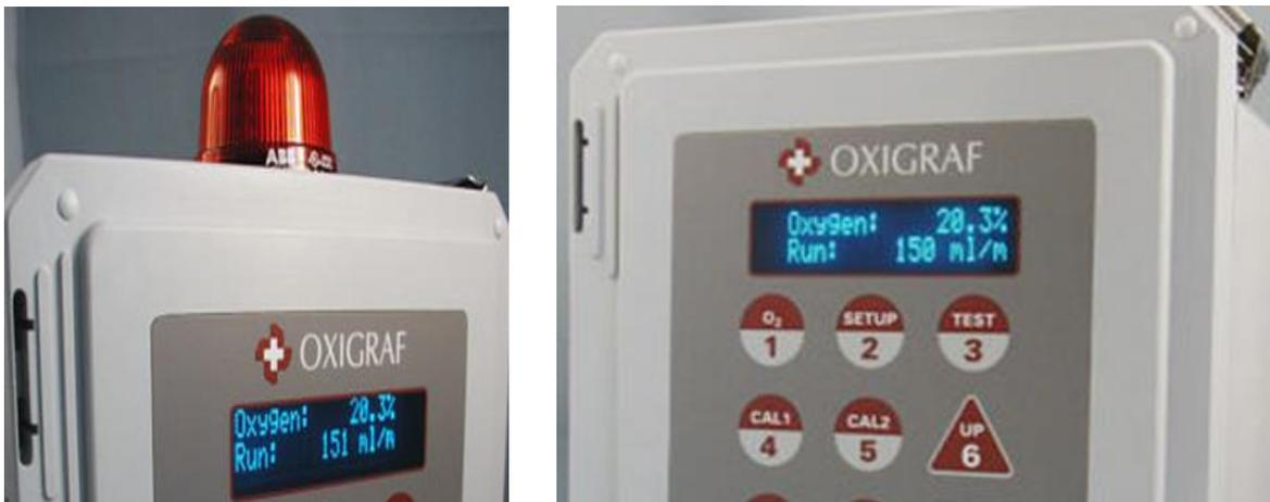
This unique sensor features a rapid response time of less than a second. The built-in pump draws gas remotely, allowing for these quick response times. In fact, we offer the best response speed/signal in the industry, and can add multiplexors (valving) in order to monitor four or more locations from over 100 feet away. The transit time of the gas sample through the sampling tube may be 1 second per meter of sampling tube with our standard pump or using our high flow option,
